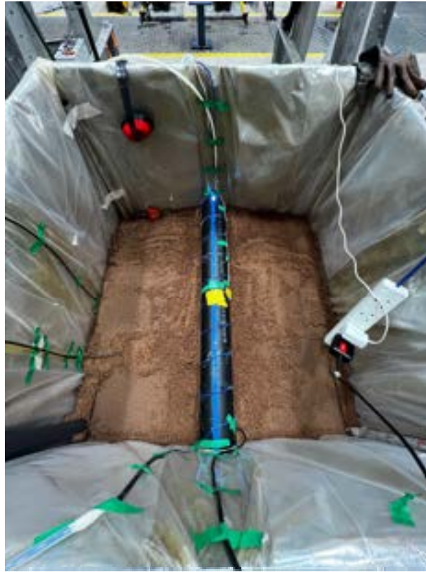
The buried pipe with 40cm cover depth
