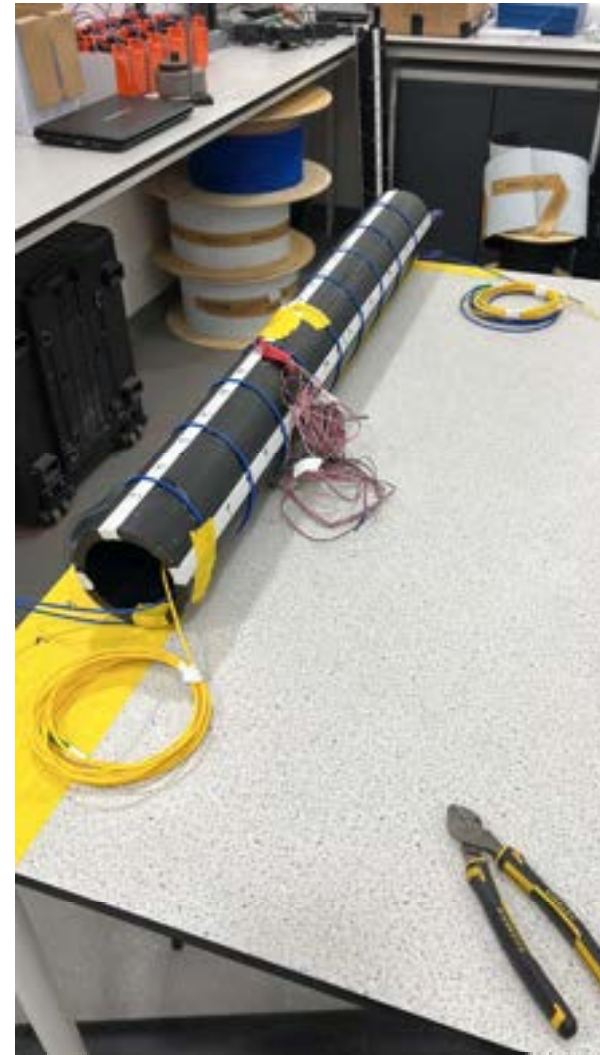
The instrumented pipe with fibre optic and strain gauges
